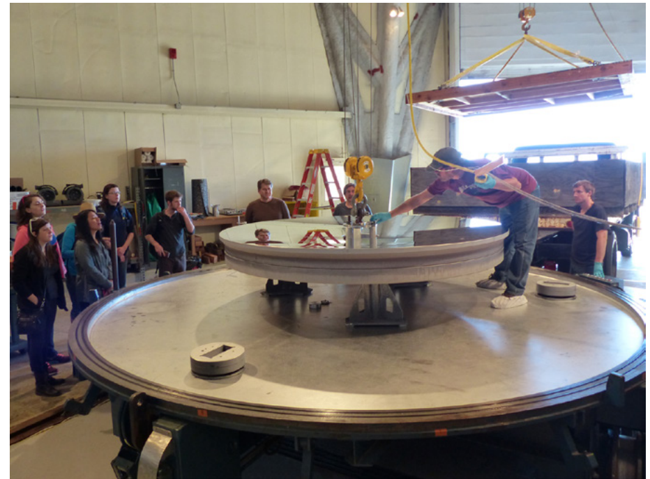
The freshly recoated 2.4-meter Hiltner mirror of the Michigan-Dartmouth-MIT Observatory sits, ready to go, at Kitt Peak's realuminization facility. [Sally Oey/U. Michigan]
